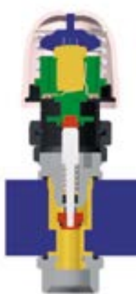
Type NC: Valve closed
